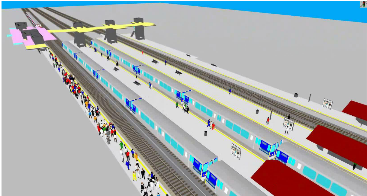
Figure 1: For the simulation of North Melbourne Station considerable effort has been put to collect data for a calibration of the simulation to reproduce the situation as it is today (Laufer, 2008).
