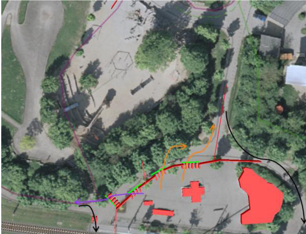
Figure 7: The first simulations showed that with the assumed origins, routes, and destinations counterflows immediately in the back of the ticket gates would occur (upper image, the visitors enter from the lower right and have to pass through the half circle of security checks). This was estimated to be realistic, as it was assumed that the visitors would not automatically and also not with information and invitations align into the right queue according to where they want to go later. Therefore an additional barrier was placed behind the gates (lower image) that prevented counterflows from occurring. This had the consequence that it had to be guaranteed that all visitors aligning at S1 (the left-most security check) were ticket owners, as they only could progress through a ticket gate and access to the free area was not possible.
