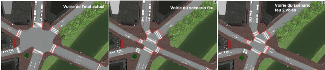
FIGURE 8: Current situation (left, “Voirie de l'état actuel”) and two alternative scenarios (center and right). The two alternatives differ in their signal programs (“feu”) and in that in the second alternative scenario there is a right turning lane for the vehicles leaving the bridge (“2 voies”). An animation of a simulation run of the current state can be seen here: http://youtu.be/YzPYwfHe0VU . The 3D visualization of the buildings of the environment is one single 3D model which has been loaded as background into the simulation software. This is not a requirement for the simulation.
